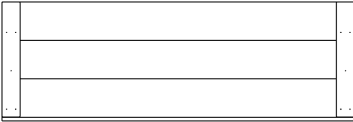
RP1 | PANEL DE TECHO - W104015 (x1) | 1 5/8"x15 5/8"x46" (42x396x1168)
